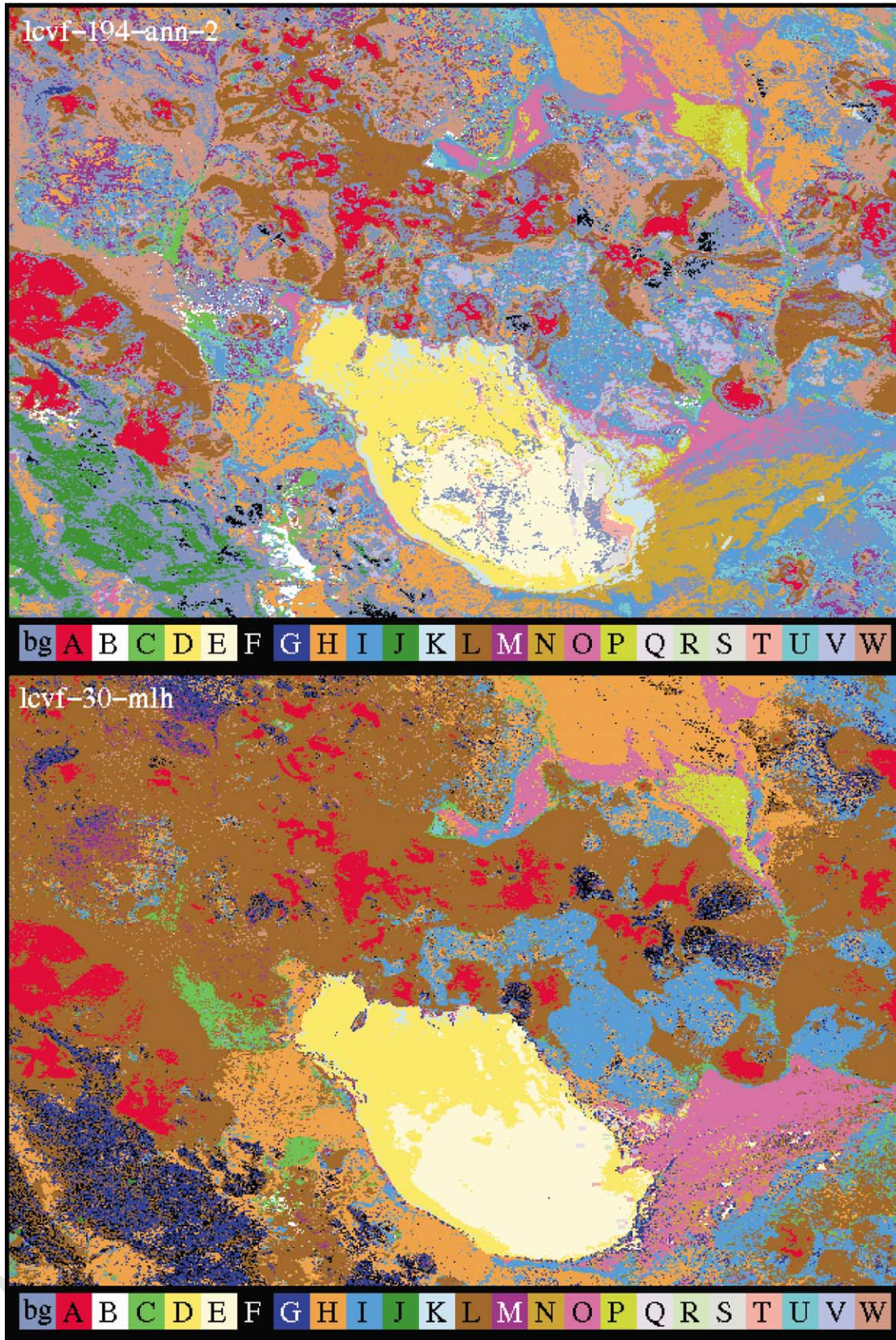
Fig. 7. Top: SOM-hybrid supervised ANN classification of the LCVF scene, using 194 image bands. The overall classification accuracy is 92% (Merényi et al., 2001). Bottom: maximum likelihood classification of the LCVF scene. 30, strategically selected bands were used due to the limited number of training samples for a number of classes. Considerable loss of class distinction occurred compared to the ANN classification, resulting in an overall accuracy of 51%. 'bg' stands for background (unclassified pixels).
