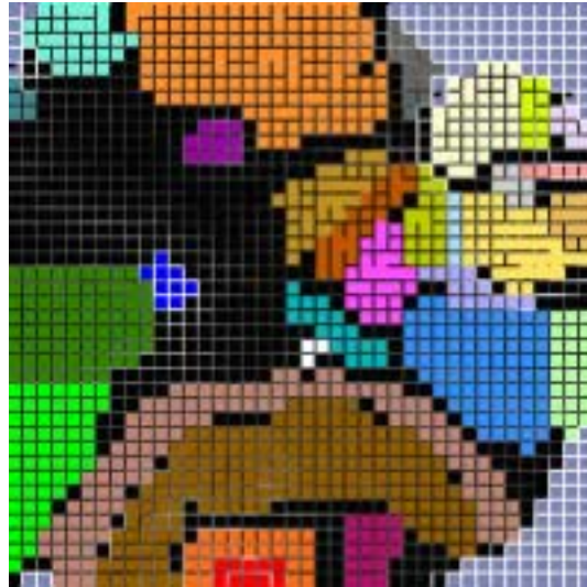
Fig. 4. Clusters identified in a 40 x 40 SOM. The SOM was trained on the entire 194-band LCVF image, using the DeSieno [22] algorithm.
