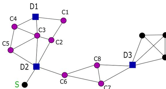
Figure 4.2: Set of dominators and connectors in DCCB scheme. The broadcast packet can reach  $D1$  through the paths  $D2 \rightarrow C3$ ,  $D2 \rightarrow C5 \rightarrow C4$  and  $D2 \rightarrow C2 \rightarrow C1$ .
