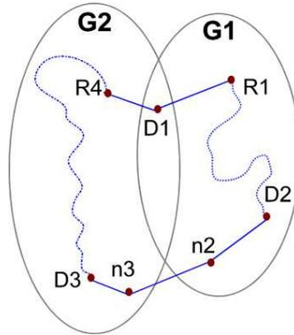
Figure 7.2: Failure of  $D1$  causes a global disconnectivity over the backbone ( $D1$  is a bridge for the backbone subgraph).
