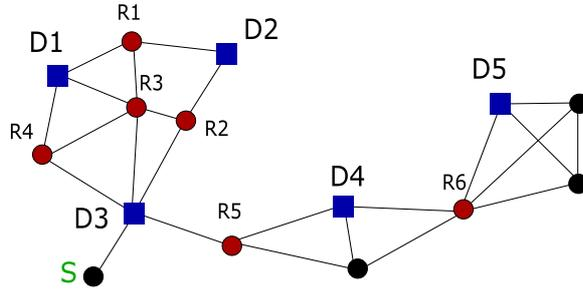
Figure 4.1: Set of dominators and reflectors for DRB scheme. The broadcast packet can reach  $D2$  through the paths  $D3 \rightarrow R2$ ,  $D3 \rightarrow R3 \rightarrow R1$  and  $D3 \rightarrow R4 \rightarrow D1 \rightarrow R1$ .
