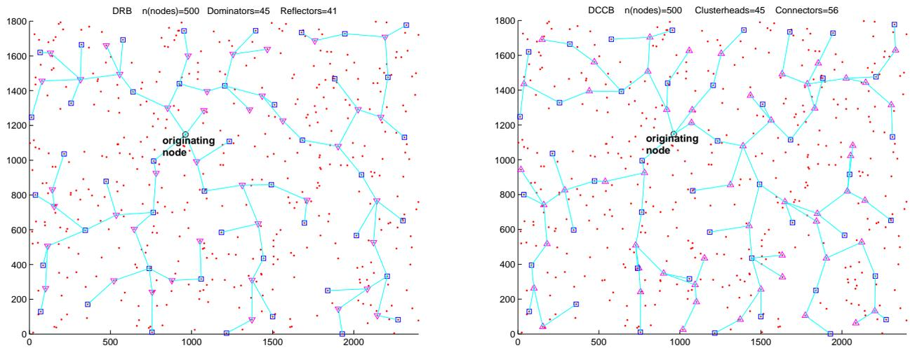
Figure 4.3: Generated random spanning tree for a broadcast packet by DRB and DCCB schemes in a homogeneous network.
