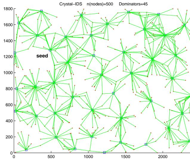
Figure 3.1: A simulation of a network with uniformly distributed nodes. Note that the Independent Dominating Set (IDS) generated by the crystal-DS algorithm is well-spread within the network. Several domantee nodes can act as reflectors between pairs of dominators.
