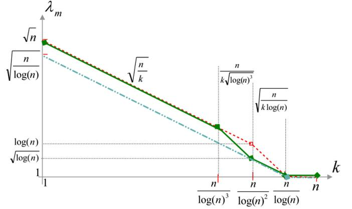
Fig. 4. Lower bound on multicast capacity in terms of  $k$ . The lower line represents multicast capacity for Protocol Model 3 and the upper line shows the capacity bound for the other channel models.
