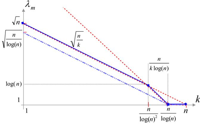
Fig. 3. Upper bound on multicast capacity in terms of  $k$ . The lower line represents multicast capacity for Protocol Model 3 and the upper line shows the capacity bound for the other channel models.
