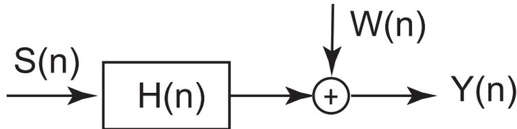
Figure 1.5: System representation of a communication channel.
