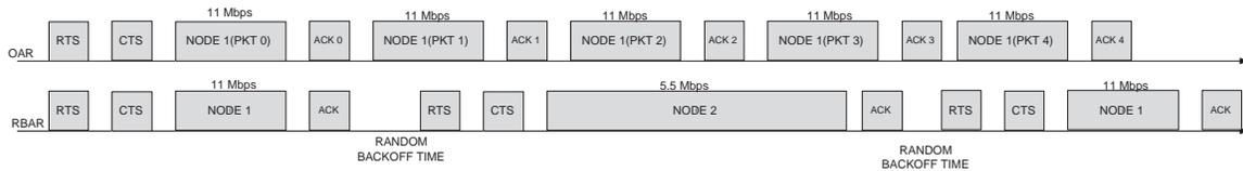
Figure 1.9: Illustration of OAR and RBAR Time-lines for a two node system. Node 1 is in a better channel state than node 2 (11 versus 5.5 Mbps).
