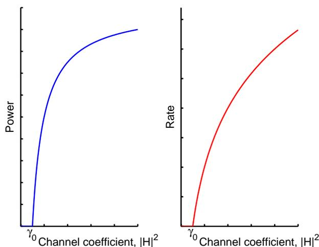
Figure 1.6: Power and rate adaptation based on channel condition for maximizing throughput.
