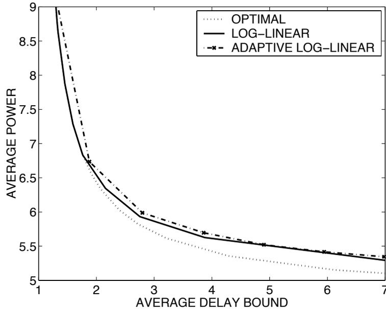
Figure 1.2: Comparison of log-linear and adaptive log-linear schedulers with corresponding optimal scheduler (Buffer length  $L = 50$ , maximum arrival  $M = 6$ , uniform arrival distribution).
