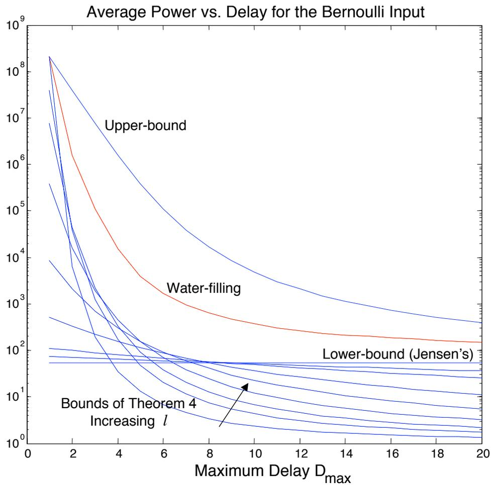
Figure 1.4: Performance of the optimal time-varying robust scheduler and the bounds on performance. Note that performance of the optimal time-invariant robust scheduler matches the upper bound.
