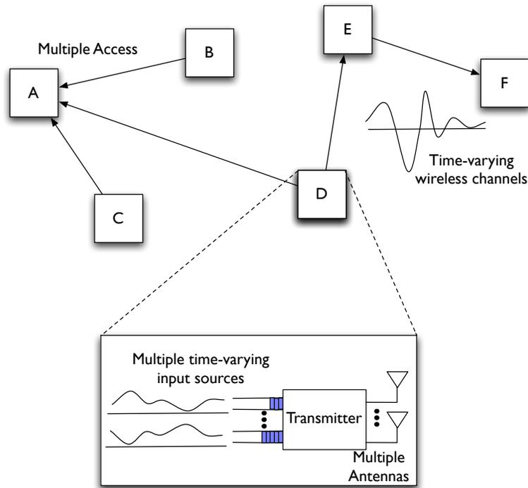
Figure 1.1: A typical multi-hop wireless network with multiple nodes. The figure also shows an expanded view of a typical node which could have multiple sources to be sent using a physical layer transmission over multiple antennas.
