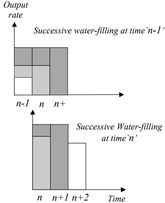
Figure 1.3: Water-filling solution for the time slot  $n - 1$  and subsequent time slot  $n$ .
