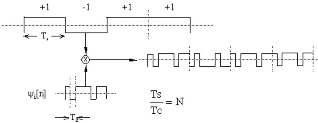
Figure 9: The spreading operation.
