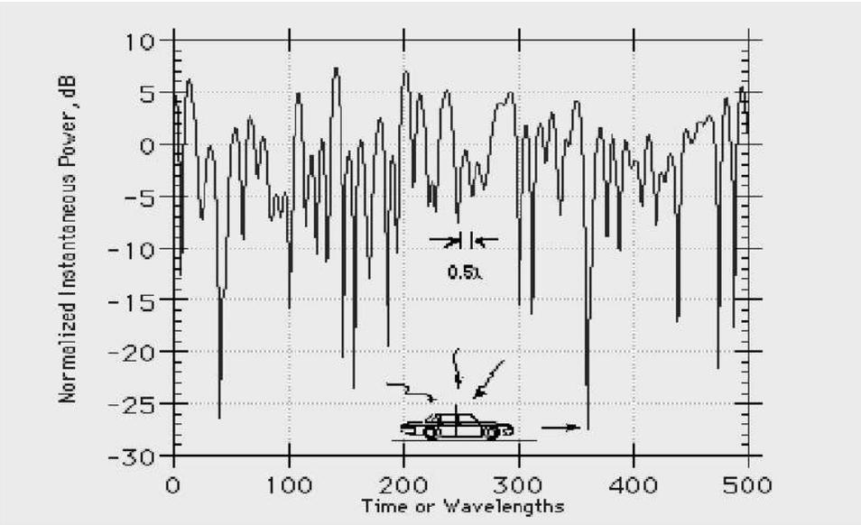
Figure 3: Time variations in the received signal power due to multipath and user mobility.
