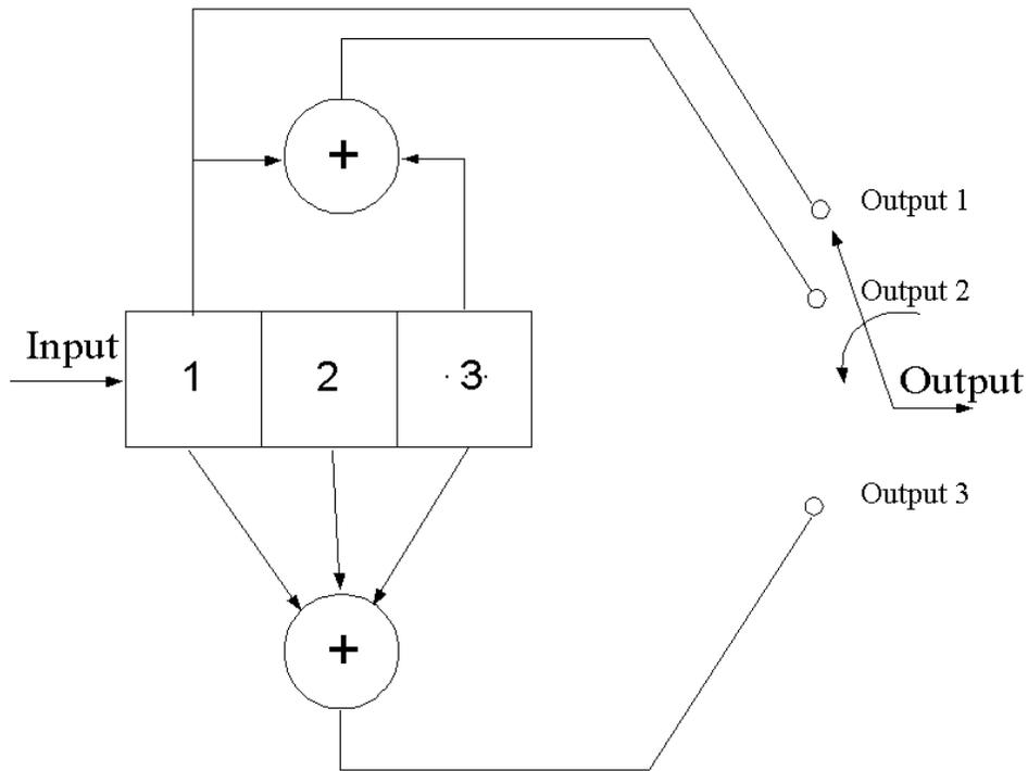
Figure 7: Convolutional encoder for a (3,1) code.
