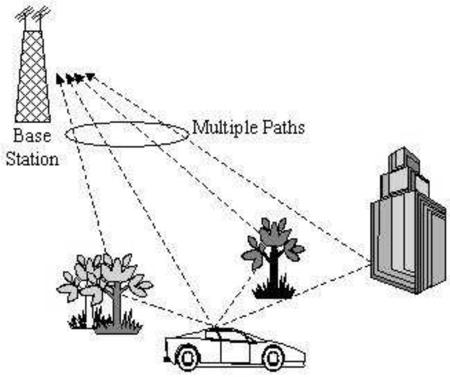
Figure 2: Multipath propagation.
