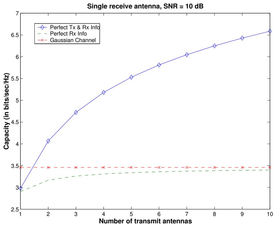
Figure 4: Capacity with multiple transmit antennas and single receive antenna, with different amount of channel state information at the transmitter.
