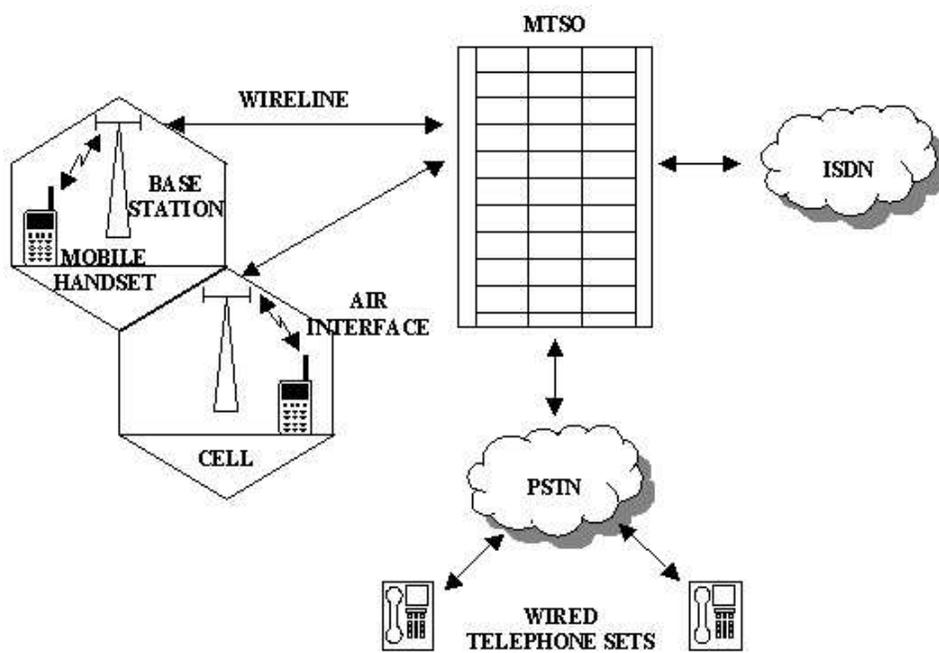
Figure 1: Components of a cellular wireless network.
