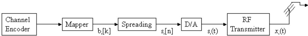
Figure 5: DS-CDMA handset transmitter components.
