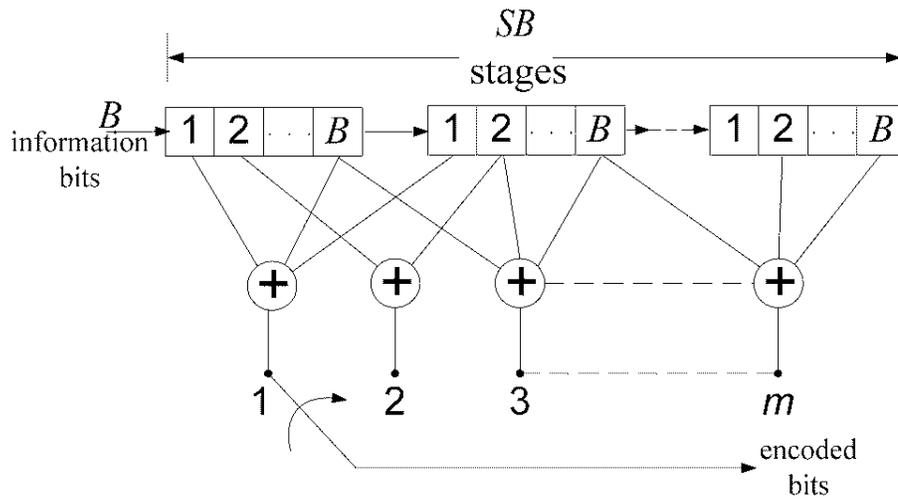
Figure 6: Convolutional encoder.
