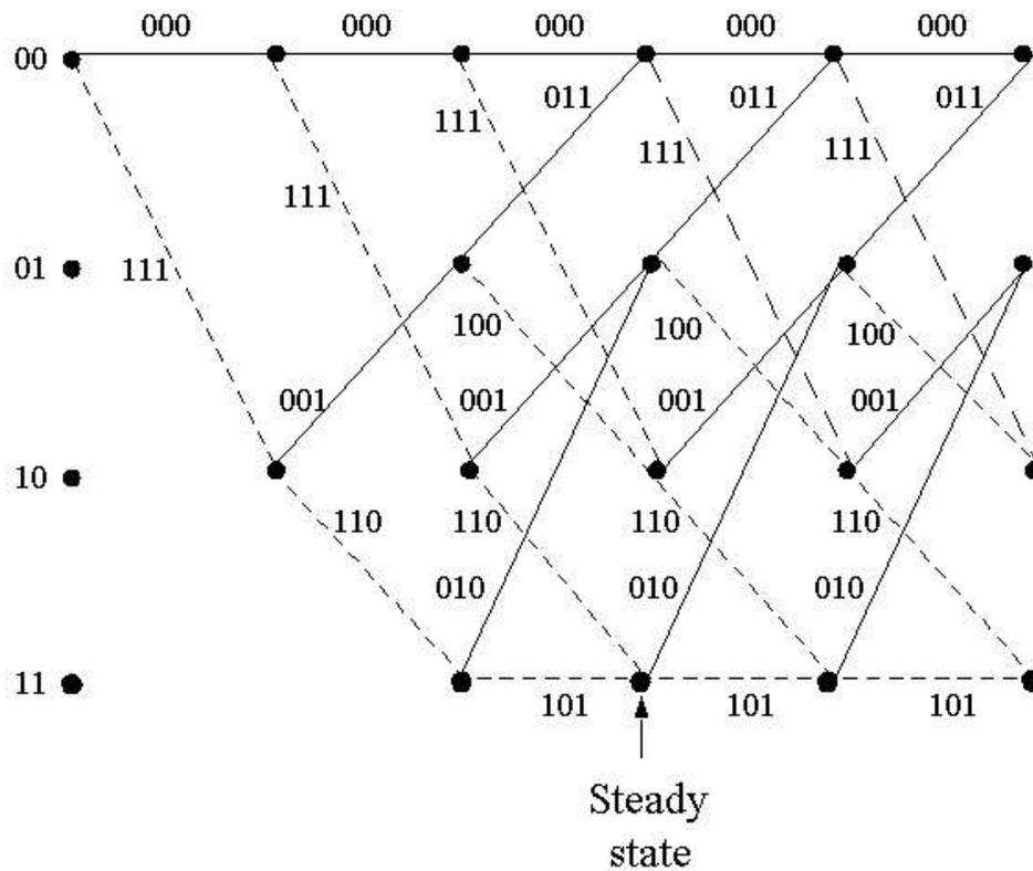
Figure 11: Trellis diagram for the example (3,1) convolutional code.
