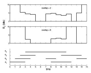
Fig. 3. Dynamic bit allocation in a two-subspace system. The top two plots depict  $B_1$ , the bit allocation to  $W_1$  resulting from maximizing  $\gamma$ . At any time each of four events may be present. For the top plot, the two feature subspaces share two common dimensions, whereas for the middle plot they share eight dimensions. In the high-overlap case, bits are more often allocated to a single subspace. The bottom plot indicates the events present at each time step.
