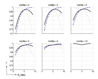
**Fig. 2.** Information transfer vs. bit allocation to one subspace for a two-feature system. Shown are the information transfer ratios for two events  $e_1$  (dashed) and  $e_2$  (dotted) with priorities  $\alpha_1 = 3/4$  and  $\alpha_2 = 1/4$ . The solid curve is the priority-weighted sum  $\gamma$ . With increasing overlap between features, allocating more bits to  $W_1$  maximizes  $\gamma$ .
