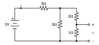
**H1.5** Find  $v_{out}$  in the circuit below.
