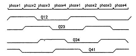
Note that Q12 and Q34 together form a non-overlapping two phase system, as do Q23 and Q41.
