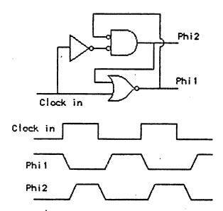
The non-overlap period must be long enough that all timing signals derived from the master clocks properly follow the two-phase discipline. There are several methods for ensuring this. The simplest is to make the
