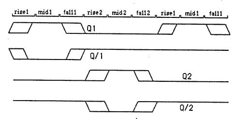
If the timing signals of a chip are labeled by class, the intervals for the six events can be found by simulation. Rise1 begins when the first Q1 signal rises (or Q/1 signal falls), mid1 begins when all the Q1 and Q/1 signals stabilize, and fall1 begins when the first Q1 signal falls or Q/1 rises. (Similarly for phase 2 signals.) The main speed limitation is that mid1 be long enough for all relevant data signals to propagate.
