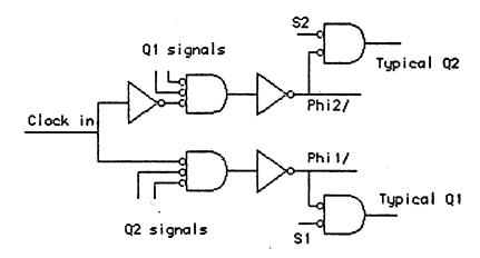
For prototypes and student projects, external two-phase clock generation is usually better than converting single-phase internally. The cost of an extra pin is irrelevant, and external clock generation adds testing flexibility. Errors in timing analysis can be more easily detected and compensated for with external clocks.
