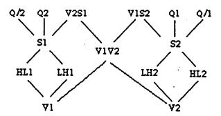
When the input to a circuit requires a signal labeled x, a signal with any label above x along the lines of the diagram may be used. However, note that Q2 and Q/2 carry no information in phase 1, and are S1 only because they are guaranteed inactive throughout phase 1. Using a Q1 signal where an S2 or V2 signal would normally be used is probably an error, since no data is carried during phase two.
