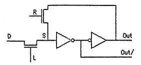
This figure shows a standard nMOS pseduo-static transparent latch. The labeling for S is the same as in the dynamic latch. New data is latched when L is high, and the old data is refreshed when R is high. Both L and R should have the same Q label (both Q1 or both Q2), but the signals are mutually exclusive, that is, L and R must never be high at the same time.
