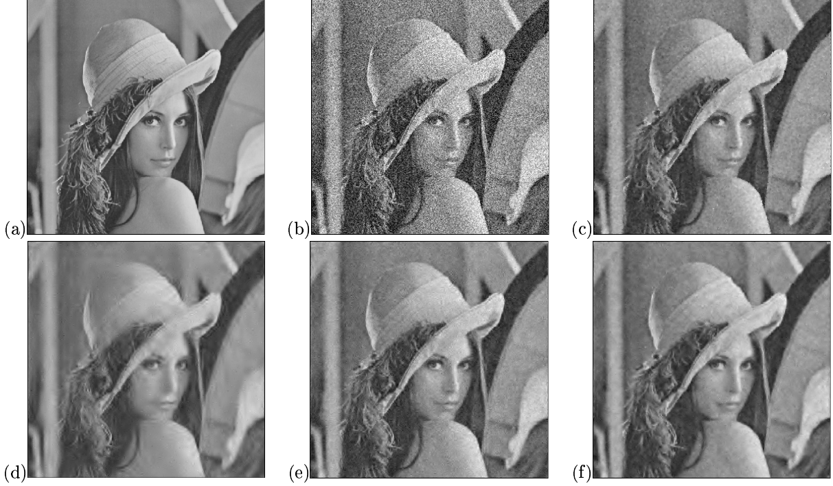
Figure 1. Image denoising examples using projections onto Besov Balls; (a) 512 \times 512 original image with 256 gray levels, (b) Noisy image ( \sigma = 35 , PSNR = 17.2dB), (c) MATLAB’s spatially adaptive Wiener filter ( 3 \times 3 window, PSNR = 27.0dB), (d) Hard thresholding in D_{12} domain using “best” threshold (PSNR = 26.1dB); the threshold was chosen to maximize PSNR, (e) Besov ball projection in B_{\infty}^1(L_1) using D_{12} wavelet (PSNR = 27.2dB), and (f) Besov ball projection in B_{\infty}^1(L_1) using 5 wavelet bases, D_6, D_8, D_{10}, D_{12} and D_{14} (PSNR = 28.3dB).
