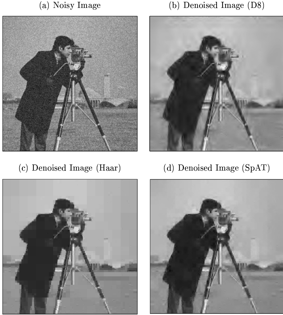
Figure 18: Top row: (a) Cameraman image with additive white Gaussian noise with standard deviation equal to 15% of the maximum image magnitude, (b) Image denoised with the Daubechies 8 orthogonal wavelet transform, 66.4941 dB PSNR. Second row: (c) Image denoised with the haar transform, 66.5983 dB PSNR, (d) image denoised with the SpAT transform, 66.8278 dB PSNR (d). The SpAT transform yields the highest PSNR while significantly reducing ringing around edges.
