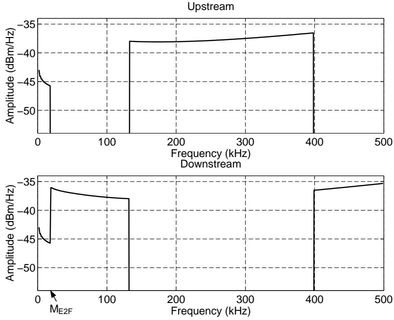
Figure 5: Optimal upstream and downstream transmit spectra for HDSL2 on CSA loop 6 with 39 self-NEXT and 39 self-FEXT interferers. EQPSD signaling takes place to the left of switch-over frequency  $M_{E2F}$  and FDS to the right. (Note that the placement of the FDS regions is nonunique. Here we choose a split such that upstream and downstream transmissions use equal transmit powers and result in equal performance margins. Other splits are possible; see [8] for details.)
