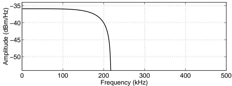
Figure 4: Optimal transmit spectra for HDSL2 on CSA loop 6 with 25 T1 NEXT interferers and AGN of  $-140$  dBm/Hz. Since there is no self-interference, FDS is not required. The upstream and downstream transmissions employ the same spectrum.
