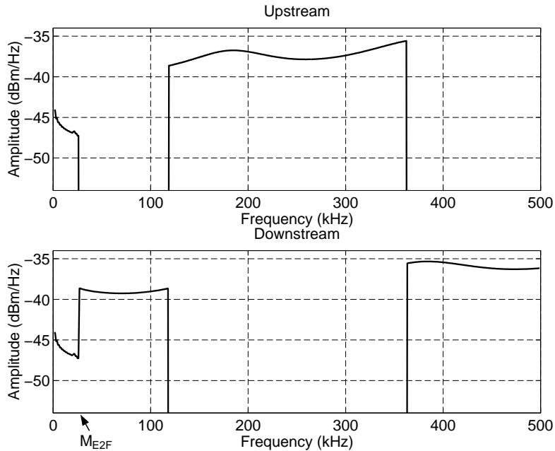
Figure 6: Optimal upstream and downstream transmit spectra for HDSL2 on CSA loop 4 with 39 self-NEXT and 39 self-FEXT interferers. EQPSD signaling takes place to the left of switch-over frequency  $M_{E2F}$  and FDS to the right. (Again we choose a split such that upstream and downstream transmissions use equal transmit powers and result in equal performance margins. Other splits are possible; see [8] for details.)
