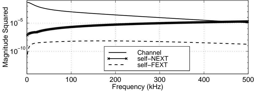
Figure 2: *Magnitude-squared transfer functions of the channel CSA loop 6 with 39 self-NEXT interferers and 39 self-FEXT interferers.*
