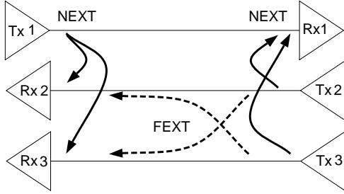
Figure 1: *NEXT and FEXT between neighboring lines in a binder. Tx's are transmitters and Rx's are receivers.*
