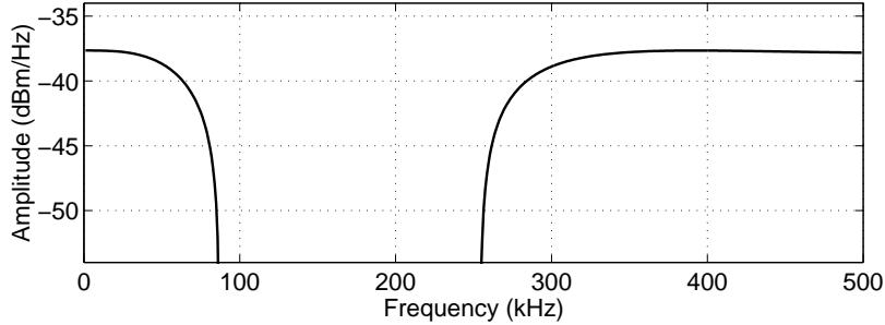
Figure 3: Optimal transmit spectra for HDSL2 on CSA loop 6 with 49 HDSL NEXT interferers and AGN of  $-140$  dBm/Hz. Since there is no self-interference, FDS is not required. The upstream and downstream transmissions employ the same spectrum.
