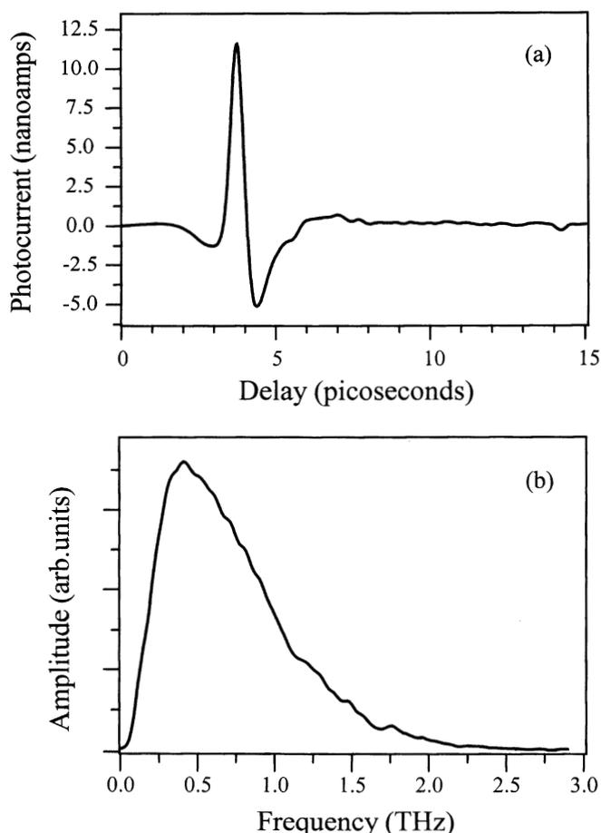
**Fig. 2a,b.** THz waveform measured using photoconductive sampling. **a** Average photocurrent (proportional to THz electric field) as a function of optical delay. **b** amplitude of Fourier transform of the signal in **a**, showing the spectral content of the radiation
