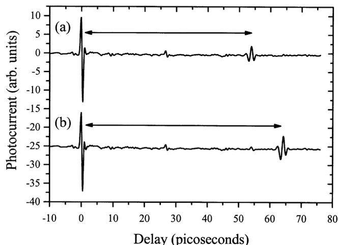
**Fig. 6.** Time-domain waveforms showing the effects of propagation through small amounts of gaseous  $\text{CH}_3\text{CN}$  (a) and  $\text{CD}_3\text{CN}$  (b). The shift in the delay of the first echo (indicated by *arrows*) results from the larger moment of inertia of the deuterated species. Waveforms offset for clarity
