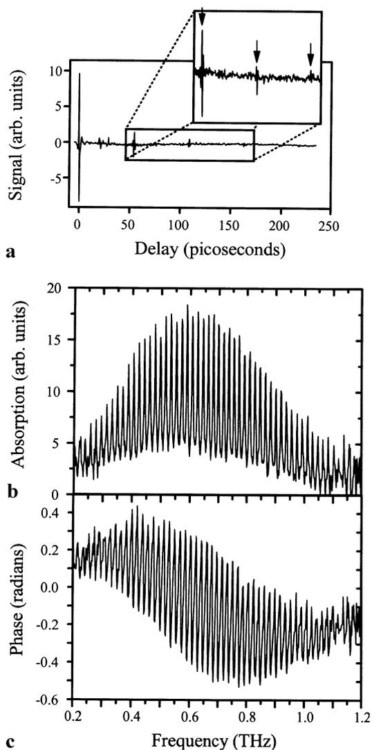
**Fig. 5.** **a** THz waveform modified by propagation through acetonitrile vapor, and the corresponding absorption (**b**) and dispersion (**c**) spectra. *Arrows* in **a** indicate the positions of the periodic echoes which result from the coherent excitation of the rotational manifold
