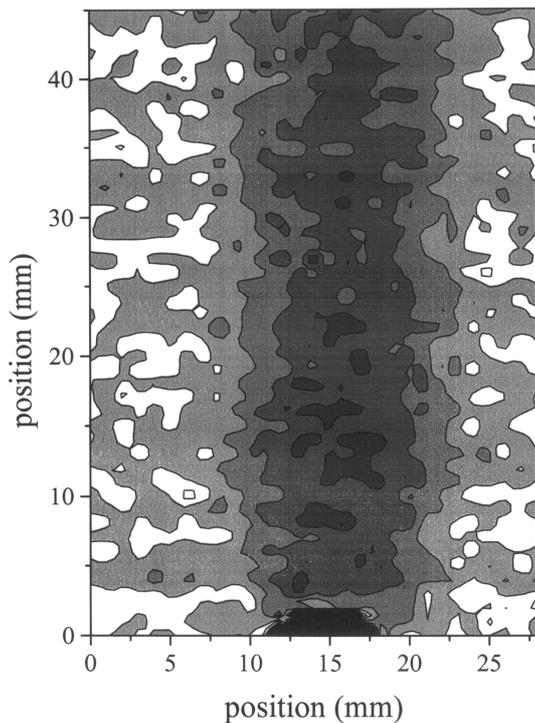
**Fig. 3.** THz image of a small gas flame, in which each contour corresponds to a shift in the transit time of the THz pulse of 5 fs. The pulse travels faster through the center of the flame because of the lower density (and thus lower index) of heated air
