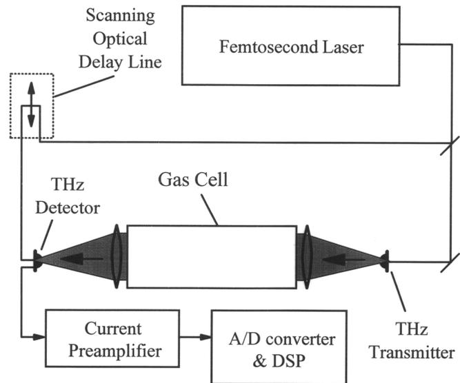
Fig. 1. Experimental setup for gas sensing measurements based on terahertz time-domain spectroscopy
