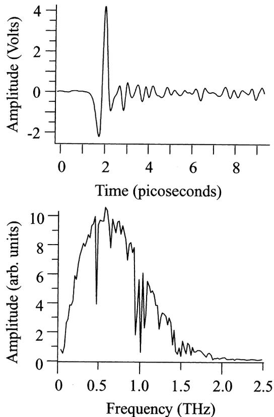
**Fig. 4.** THz waveform modified by propagation through humid air. The oscillations following the initial pulse result from the effects of water vapor. The  $\text{H}_2\text{O}$  absorption lines attenuate selected narrow frequency intervals within the spectrum of the THz pulse, as seen in the Fourier transform, at right
