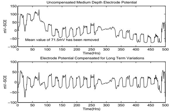
Figure 4: Compensation of Long Term Variations in Submerged Electrode
