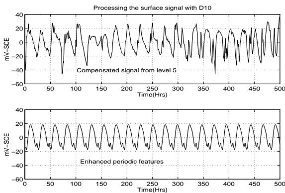
Figure 7: Enhanced Periodic Features Of The Surface Signal
