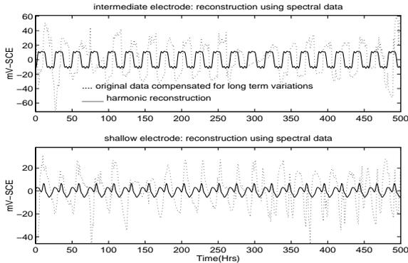
Figure 3: Harmonic Reconstruction With Four Terms
