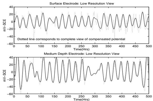
Figure 5: Low Resolution Orthogonal Components
