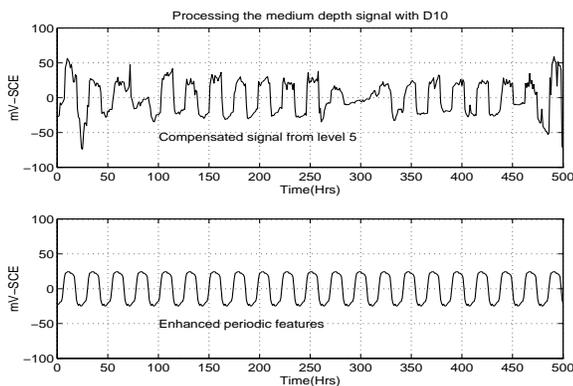
Figure 8: Enhanced Periodic Features Of The Medium Depth Signal
