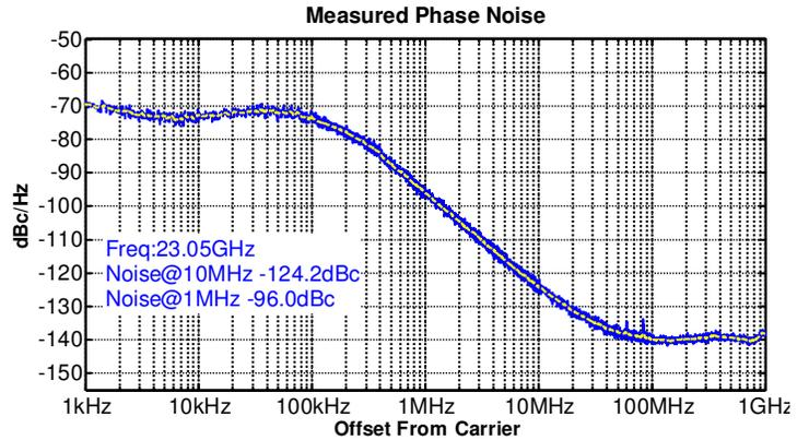
Fig. 4. Measured PLL phase noise at 23.1GHz.
