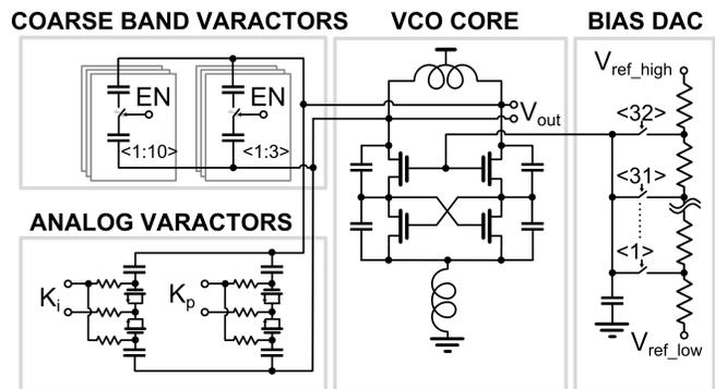
Fig. 1. Details of the modified Colpitts oscillator.
