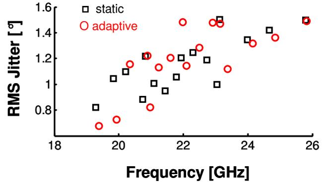
Fig. 7. Third measured RMS jitter in degree for static and adaptive bias.
