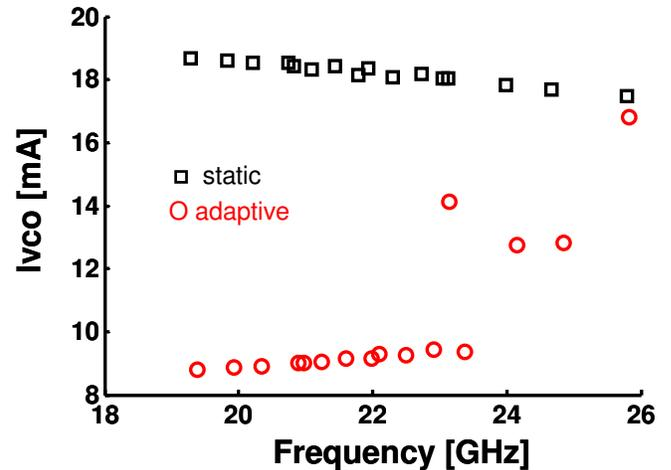
Fig. 8. Measured VCO current for static and adaptive bias.
