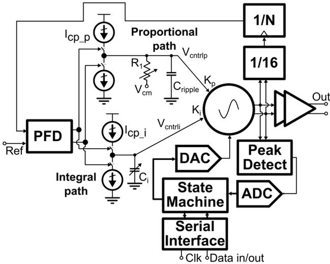
Fig. 2. Simplified PLL block diagram.
