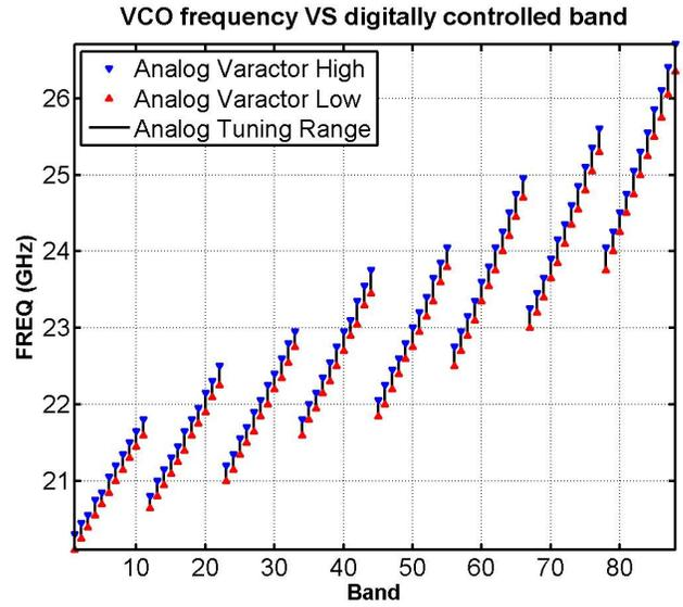
Fig. 3. VCO frequency range and band overlap.
