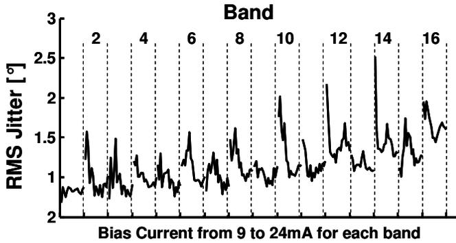
Fig. 6. Measured RMS jitter in degrees across bands and DAC settings.
