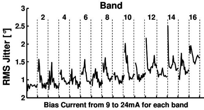
Fig. 6. Measured RMS jitter in degrees across bands and DAC settings.
