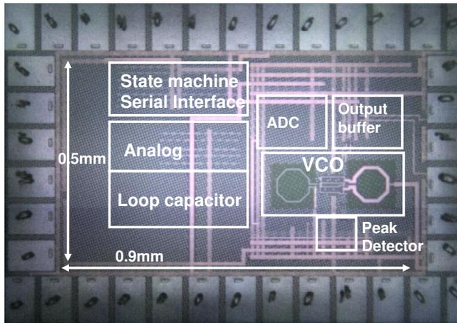
Fig. 9. Chip microphotograph.
