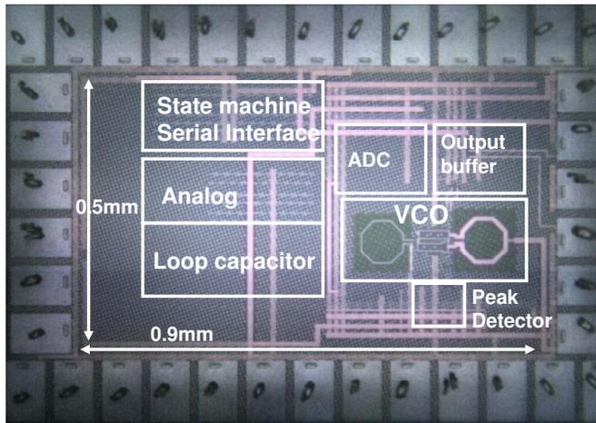
Fig. 9. Chip microphotograph.
