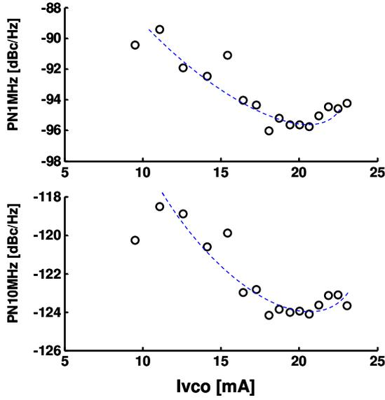
Fig. 5. 1 MHz and 10 MHz phase noise versus VCO current.
