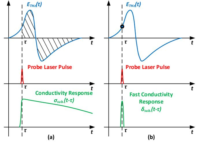
Fig. 2. Sampling mechanism of a PCA detector with (a) slow substrate conductivity response and (b) fast substrate conductivity response.
