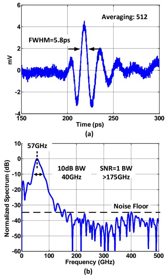
Fig. 9 (a) Measured time-domain waveform and (b) measured frequency spectrum of the picosecond pulse radiated from the chip [5].
