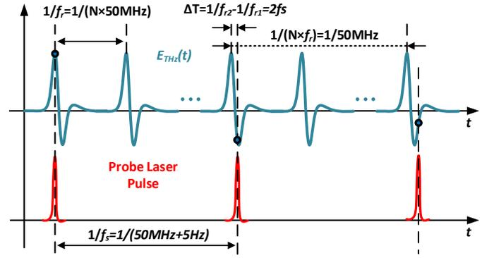
Fig. 6. Valid sampling conditions of the proposed picosecond pulse measurement technique.
