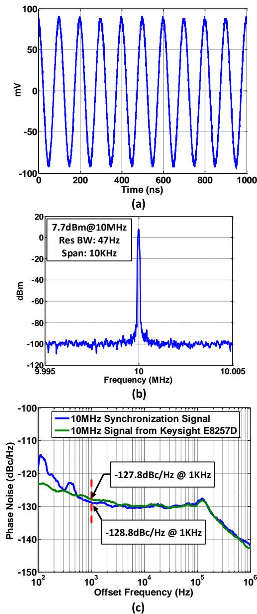
Fig. 8. (a) Measured time-domain waveform of the 10MHz synchronization signal. (b) Measured frequency spectrum of the 10MHz synchronization signal. (c) Measured phase noise of the 10MHz synchronization signal.
