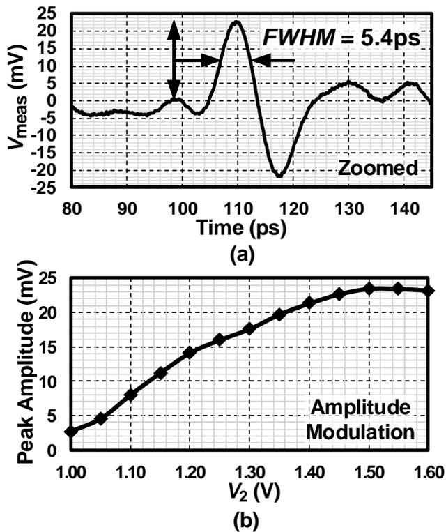
Fig. 10 (a) Measured time-domain waveform of the picosecond pulse radiated from the chip [9]. (b) Measured pulse amplitude modulation of the chip [9].
