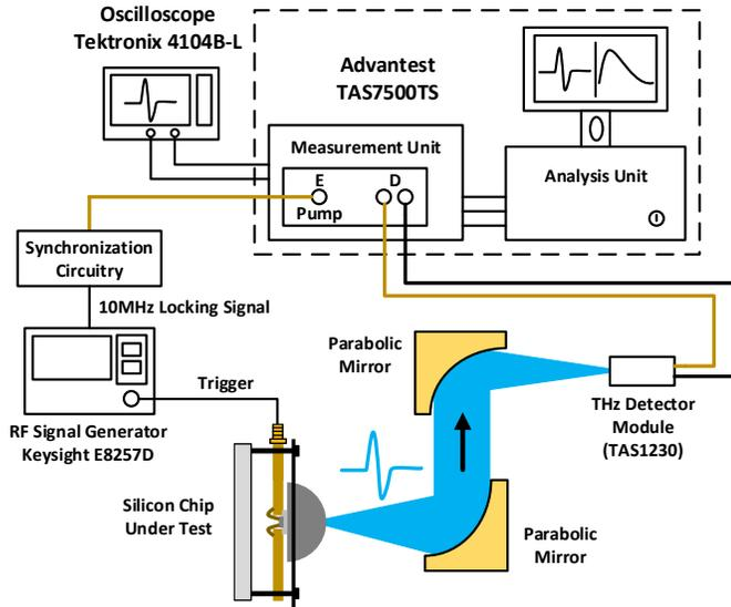
Fig. 4. Schematic of the proposed measurement technique.
