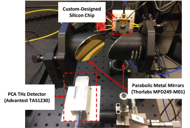
Fig. 7. Measurement setup for characterizing custom-designed silicon chips.
