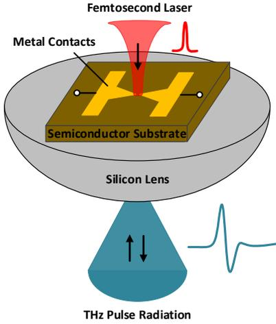
Fig. 1. Schematic of a photoconductive antenna (PCA).
