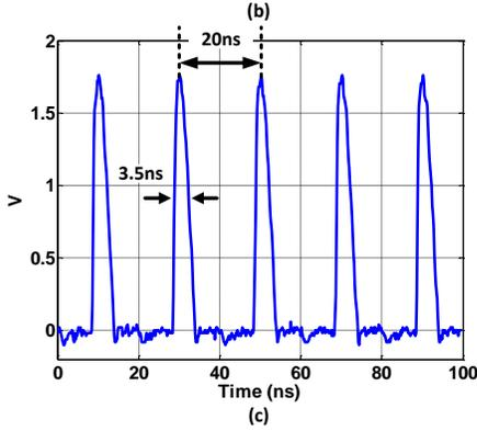
Fig. 5. (a) Block diagram of the proposed synchronization technique. (b) The actual circuit blocks for synchronization signal generation. (c) Converted electrical pulses from the pump femtosecond laser.
