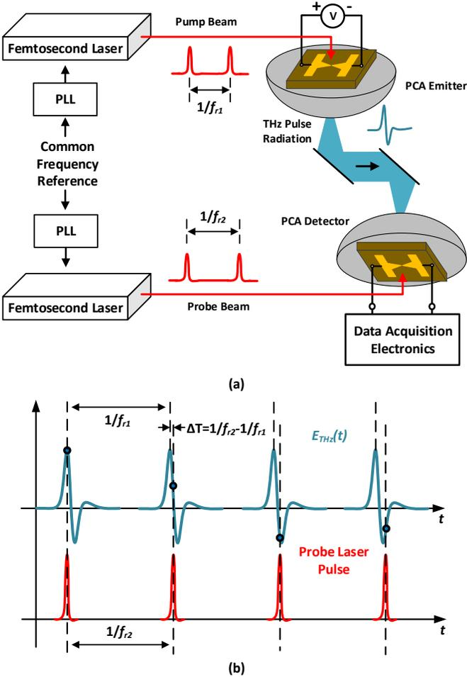
Fig. 3. (a) Schematic of a THz-TDS system with ASOPS scheme. (b) Sampling mechanism of ASOPS scheme.
