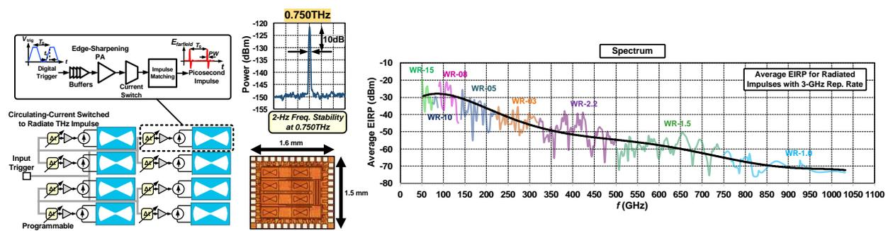
Fig. 1. Custom silicon source for radiating picosecond pulses
