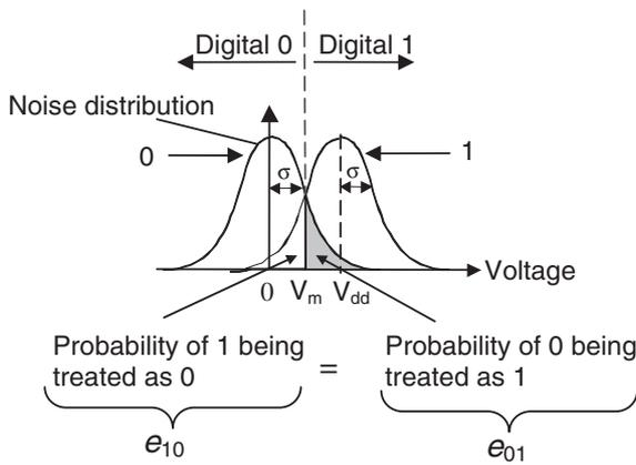
Fig. 2. The digital value 0 (and 1) corresponding to the noisy output (input) voltage of the probabilistic inverter is represented by a Gaussian distribution with a mean value of 0 (or  $V_{dd}$ ) and a standard deviation  $\sigma$  which is the rms value of the noise—modeled for both the input- as well as the output-coupled cases.
