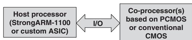
Fig. 11. A probabilistic system-on-a-chip architecture following Chakrapani *et al.*<sup>24)</sup>
