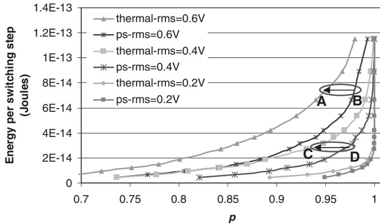
Fig. 7. Comparison of the  $E-p$  relationships in the instances of power supply noise coupling and output-coupled thermal noise.
