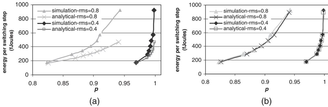
Fig. 8. The  $E$ - $p$  relationship of the CMOS inverter with the parameters shown in Table II where the analytical model (a) does not include the short-circuit energy (b) includes the short-circuit energy component.
