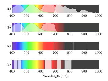
**Fig. 3. Spectral responses:** The spectral response for the various imaging modalities superimposed upon a representation of the spectrum sampled by the HSI. (a) shows the RGB and NIR spectral responses, (b) shows RGB and three narrowband filter locations (in white), (c) shows the location of the six narrowband filters (in white), and (d) shows the location and bandwidth of the six optical filters. The broadband spectral curves have been normalized for clarity.
