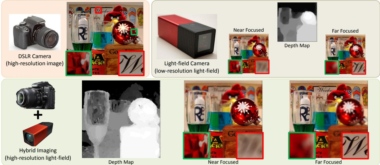
Figure 2: Traditional cameras capture high resolution photographs but provide no post-capture focusing controls. Common light field cameras provide depth maps and post-capture refocusing ability but at very low spatial resolution. Here, we show that a hybrid imaging system comprising of a high-resolution camera and a light-field camera allows us to obtain high-resolution depth maps and post-capture refocusing.
