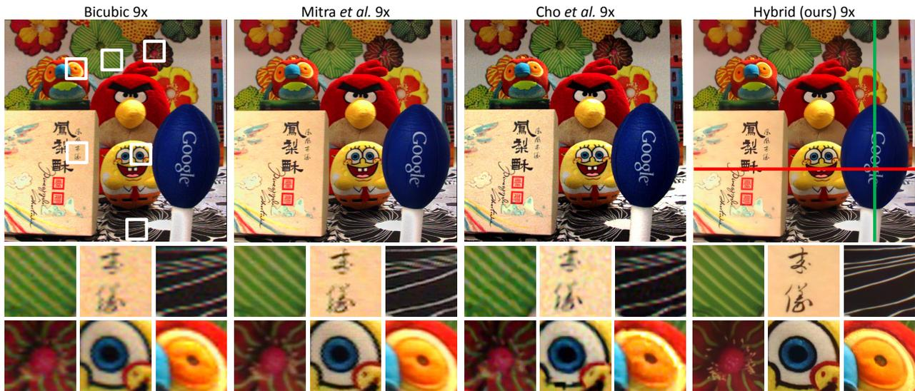
Figure 4: *9× LF super-resolution of a real scene*: The scene is captured using a Lytro camera with a spatial resolution of  $380 \times 380$  for each view. We show the central view of the  $9\times$  super-resolved LF, reconstructed using bicubic interpolation, Mitra *et al.* [27], Cho *et al.* [11], and our algorithm. As shown in the insets, our algorithm is better able to retain the highly textured regions of the scene.
