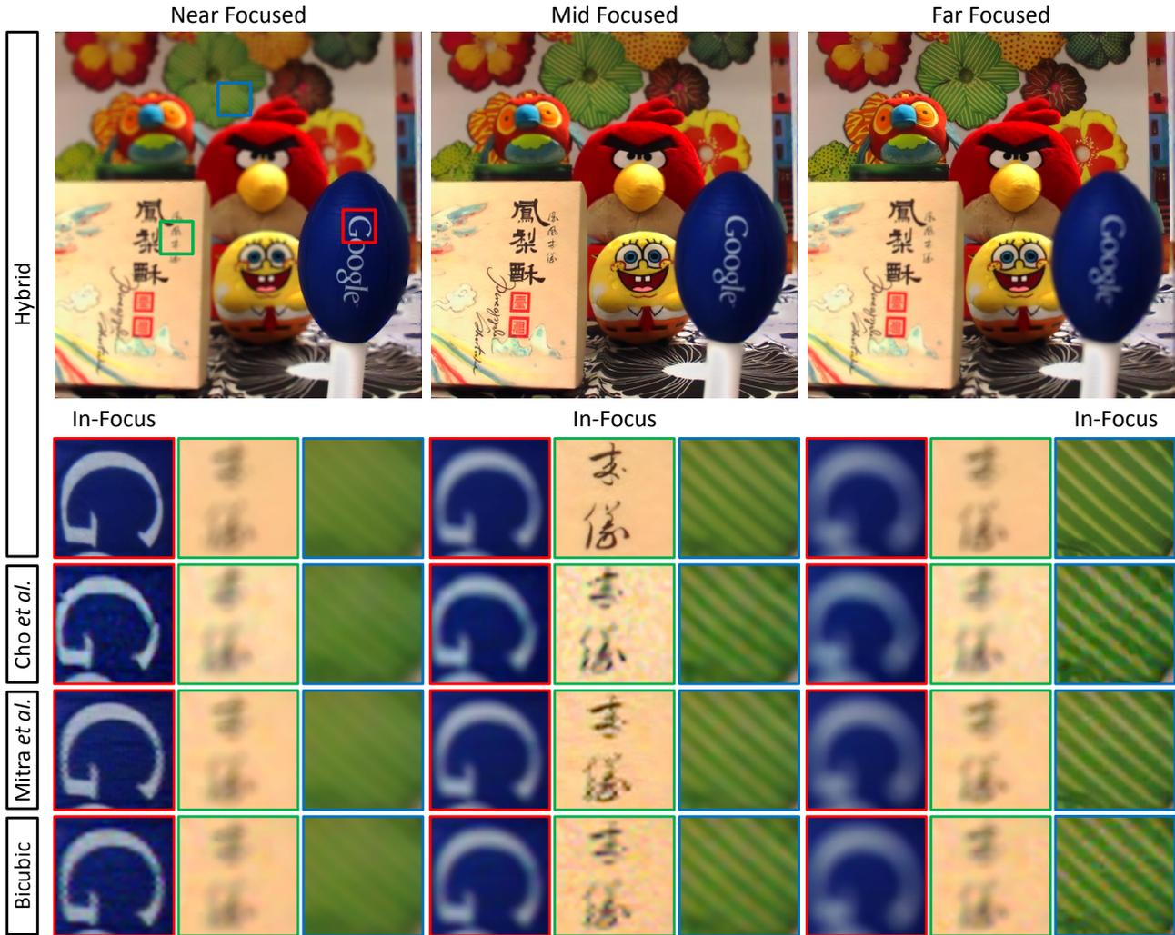
Figure 8: *Refocusing results for real scene*: On the top, we show the LF super-resolved using our method refocused at different depths. Below that, we show zoomed insets from refocused results produced by bicubic interpolation, Mitra *et al.* [27], Cho *et al.* [11] and our algorithm. The focused region produced by our algorithm are much more detailed compared to other results.
