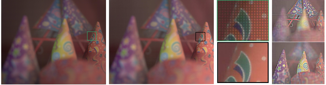
Figure 5.8: Our heterodyne light field camera provides 4D light field and full-resolution focused image simultaneously. (First Column) Raw sensor image. (Second Column) Scene parts which are in-focus can be recovered at full resolution. (Third Column) Inset shows fine-scale light field encoding (top) and the corresponding part of the recovered full resolution image (bottom). (Last Column) Far focused and near focused images obtained from the light field.
