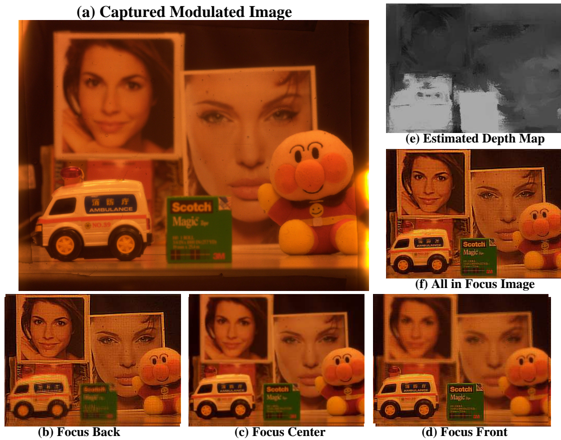
Figure 5.14: (a) Captured Modulated Image (b) Refocused Image - Focus on back poster (c) Refocused Image - Focus on doll (d) Refocused Image - Focus on front Scotch box (e) Raw Depth labels quantized to 10 depth levels. (e) All in focus image.
