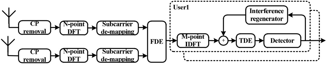
Fig. 1. LTE uplink MIMO receiver with interference cancellation
