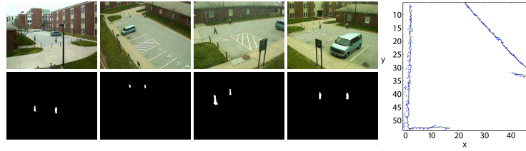
Fig. 5. Tracking results on a video sequence of 300 frames. ( Left ) The first two rows show sample images and background subtraction results using the compressive measurements, respectively. The background subtracted blobs are used to detect target location on the ground plane. The right figure shows the detected points using CS (blue dots) as well as the detected points using full images (black). The distances are in meters.
