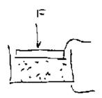
The inconsistency and noise caused by the shifting of the carbon granules can be eliminated by imbedding them in an elastomer such as rubber, which holds them in a fixed relationship to each other, but still allows local deformation at the points of contact.
