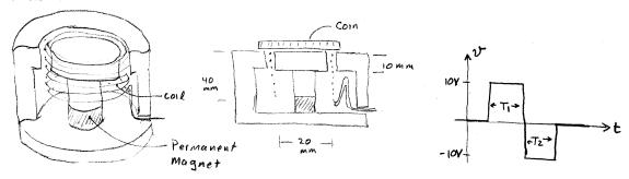
A coin is tossed by applying a short 10 V pulse to the coil. To prevent the coil from being tossed along with the coin, this pulse is immediately followed by a -10 V pulse to decelerate the coil and return it to its starting position. The composite tossing pulse is shown in the plot below. The coin being tossed is a US Quarter Dollar.
