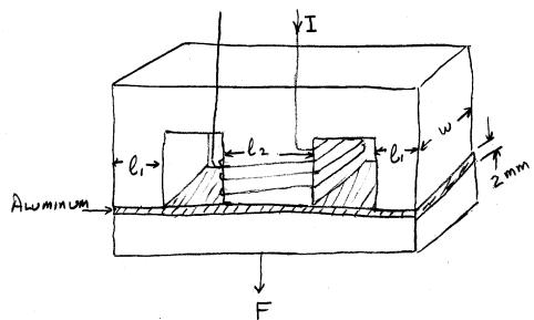
**H8.3** The electromagnet shown in the figure exhibits linear  $\lambda$  vs. i behavior until it abruptly saturates. The relation between  $\lambda$ , i, and x is given by the equations
