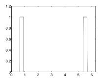
Now consider another magnitude frequency response depicted below. This frequency response was generated using a two-pole IIR filter (two conjugate symmetric poles and two zeros at the origin).
