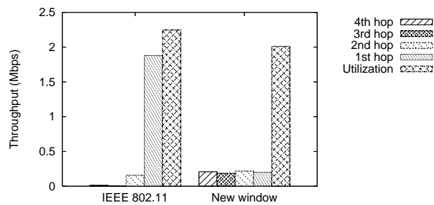
Fig. 36. TCP throughput in a four-hop chain topology, with minimum contention windows all 32 (left) and the one hop neighbor changed to 128 (right).
