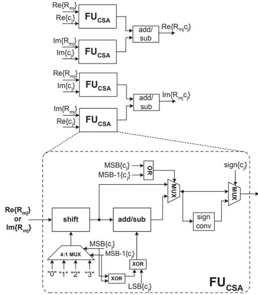
Fig. 6. Block diagram of arithmetic logic for computation of  $R_{mj}c_j$  for a single value of  $j$ . Block diagram of the  $FU_{CSA}$  for computation of partial  $R_{mj}c_j$  products: support for both 16-QAM and 64-QAM.
