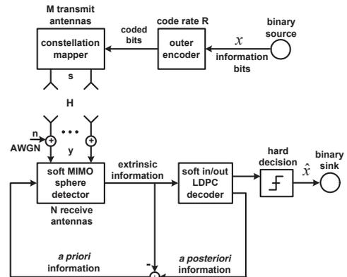
Fig. 1. MIMO transceiver, iterative detection and decoding.
