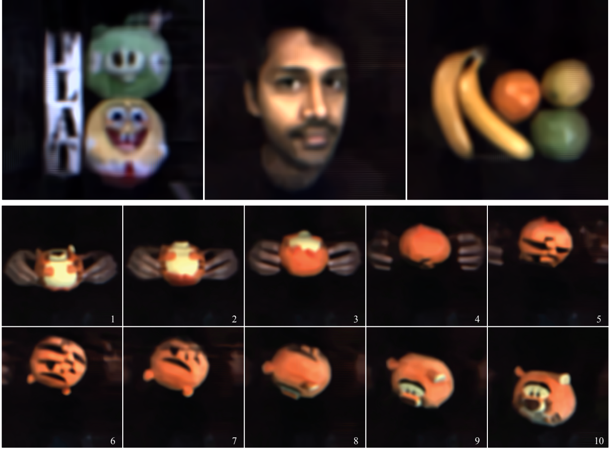
Fig. 5: (Top) Reconstruction of three static scenes using the Flea FlatCam prototype. (Bottom) Sample frames from video reconstruction of a toy performing a backflip aided by human hands. The video was recorded at 60 frames-per-second.
