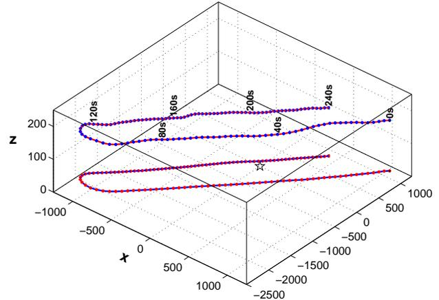
**Fig. 2.** The acoustic node (star) is situated at the origin. The calibration helicopter completes two sorties around the node for the calibration, corresponding to a four-minute run. The actual helicopter track as well as its projection on the  $x$ - $y$  plane are shown.
