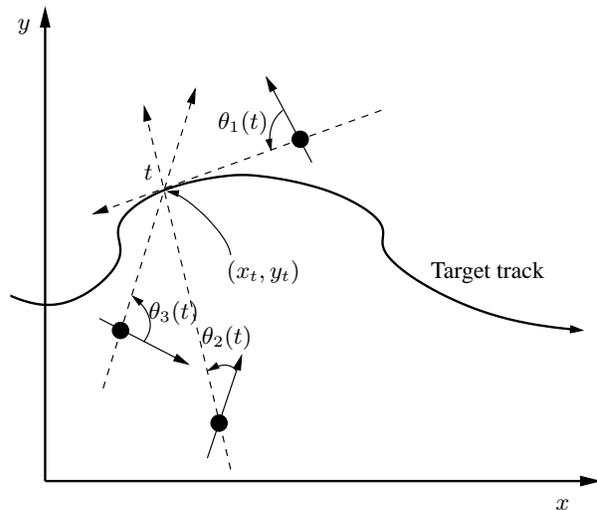
**Fig. 1.** Black dots are the acoustic nodes (arrays) and the solid arrows through the nodes represent their reference orientations for the local DOA estimates. The DOAs are measured counter-clockwise. If the node positions are known, then it is possible to determine the target position  $(x_t, y_t)$ .
