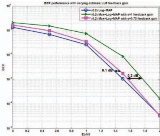
Figure 7 Simulation Result for Extrinsic LLR Scaling Method
