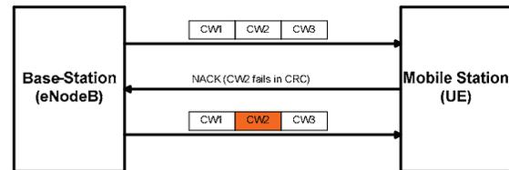
Figure 9 Example Case for Failed Data Transmission.
