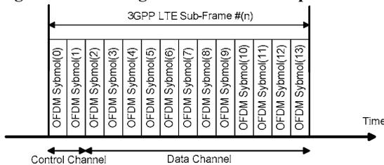
Figure 5 A 3GPP LTE sub-frame example where 2 OFDM symbols are allocated on control channel
