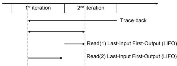
Figure 4 Tail-biting Viterbi Decoder Top-level Control
