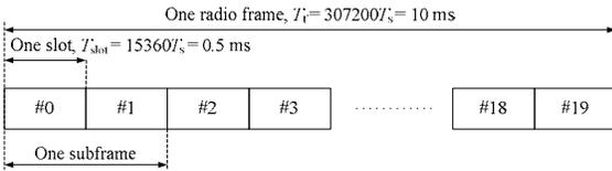
Figure 1 3GPP LTE Downlink Frame Structure [1]
