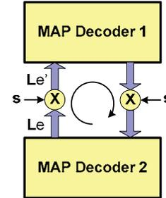
Figure 8 Extrinsic Log-Likelihood Ratio (LLR) Scaling Method
