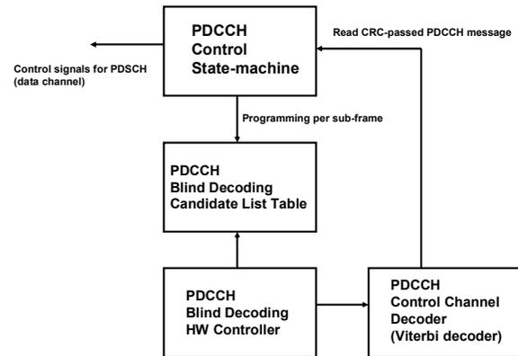
Figure 3 Data-path for 3GPP LTE PDCCH Blind Decoder
